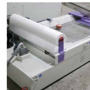
__ automatic water filtration system provides an autonomous renovation and monitoring of the filter paper's cleanliness
