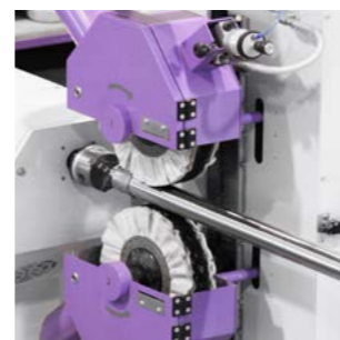
__ the machine is equipped with two stations contributing to a faster tube polishing, with tube internal supports for a scratch-free process
