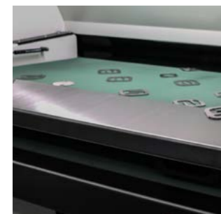
___ single sided small parts processing down to 50x50mm thanks to an additional conveyor and support table
