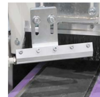
__ air blower: reducing the quantity of splashes outside of the machine
