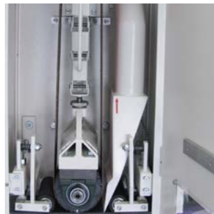
__ FC120 Z has one abrasive belt unit
